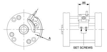
To sense piston position mount switch along tie rod using 2 each small set screws.
